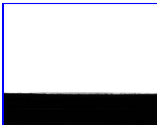
Figure 7. Oil (rapeseed) droplet shape on the nanocolumn array. The oil contact angle becomes 0^\circ 0.5 s after it was dropped onto the surface.
